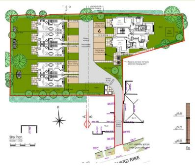
The access road to the proposed site is via Orchard Rise which is width ≈5m and length ≈105m from the Orchard Avenue/ Orchard Way intersection and thence via a narrow driveway of width ≈3m and length of ≈28m to a blind corner onto the site.
