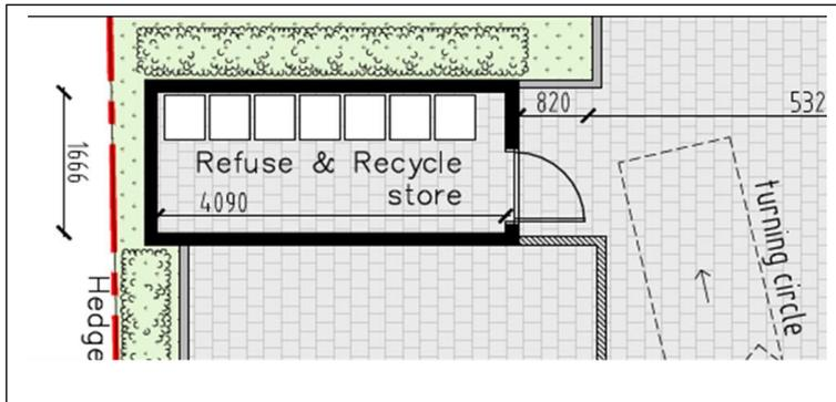
It is also understood that the access doors to the bin storage must **not open outward** over a **public footway or road**, and should **not** cause any **obstruction** to other accesses when in an open position. The proposed development Refuse Storage doors **DO open outwards** and **DO obstruct**
