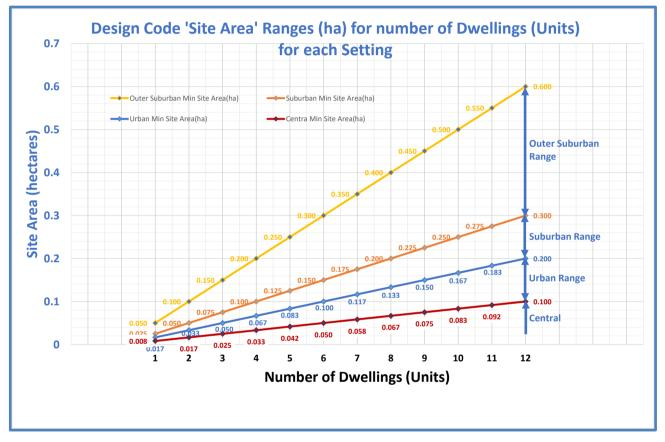
This graphical illustration demonstrates the appropriate "Site Areas" required to be within the Max & Min Ranges for each of the "Settings" (Area Types) as defined in the National Model Design Code & Guidance. We have shown the incremental number of Units (Dwellings) from 1 to 12 but the graph could be extended proportionately.
