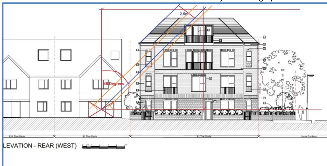
New Estimated position of French windows at the rear ground floor of 83 The Glade and the revised 45-Degree Projection after further investigation
