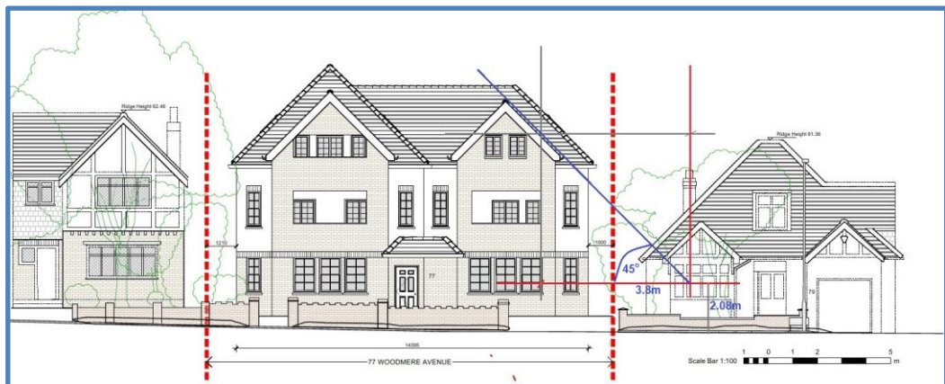
Estimated (scaled off the supplied amended drawings), the non-compliance to the 45-Degree (Vertical) Rule.
