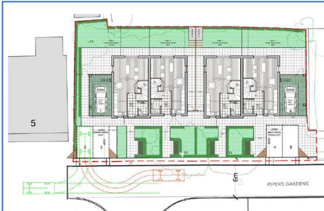
Vehicle 2 Exit encroaches over end of public Road onto Private Driveway of #5 Pipers Gardens
