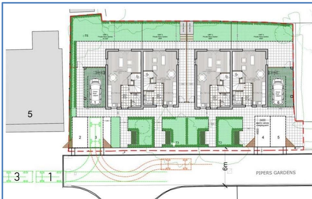
For Exiting vehicle #1, vehicle #3 must reverse onto the Private Driveway of #5 Pipers Gardens in order for Vehicle 1 to reverse out following the same path onto the private drive of #5 Pipers Gardens before exiting.
