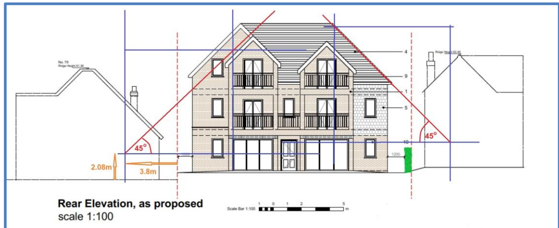
Illustration of 45° Rule vertical from the Centre of the nearest Ground Floor Window/Door of 79 Woodmere Avenue ( Distances provided by the Occupant ) fails to meet the requirement.
