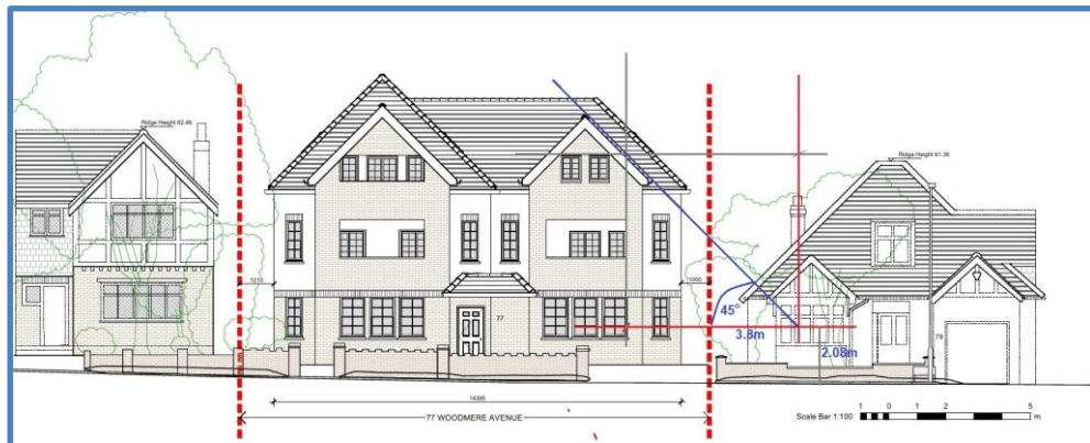
Estimated non-compliance to the 45-Degree (Vertical) Rule of SPD2 at Paragraph 2.11c.
