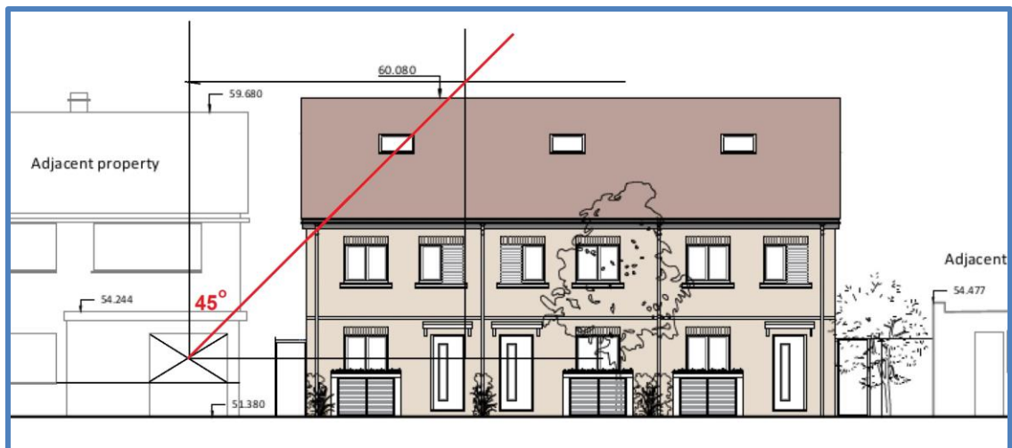
Estimated of 45° Vertical projection from centre of nearest ground floor (Rear) window of 11 Gladeside intersecting the proposed development
