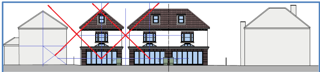
Rear Elevation indicating the separation between the proposed Semi-detached and Detached dwelling is inadequate and fails the Policy.
