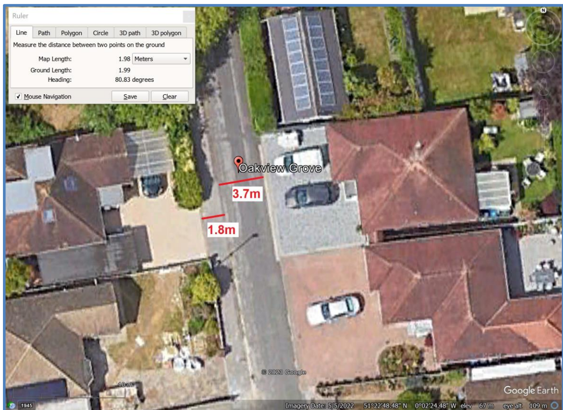
Google Earth image of Oakview Grove showing width of access road and footpath (One Side only)
