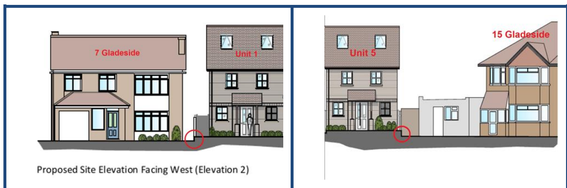
Illustration of ≈300mm to 600mm raised AOD which would result in surface water flow toward neighbouring dwellings.
