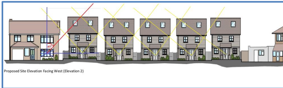
The 45-Degree projection (Vertical) from 7 Gladeside projection intersects Unit 1 & separation between Units.
