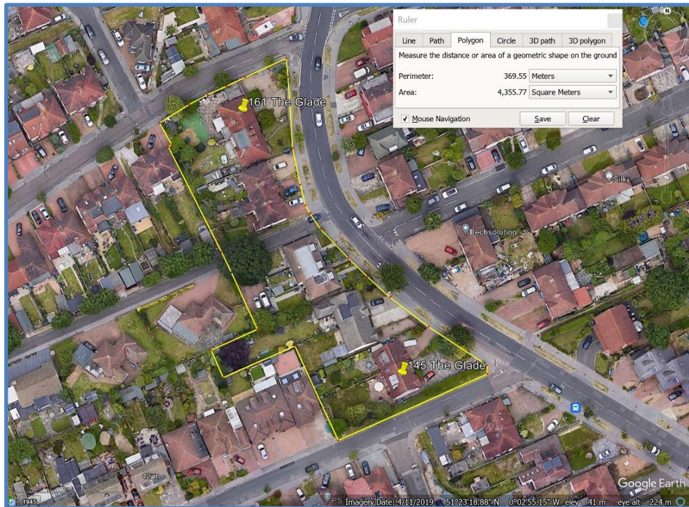
Area of Post Code CR0 7QR as measured from Google Earth Image
